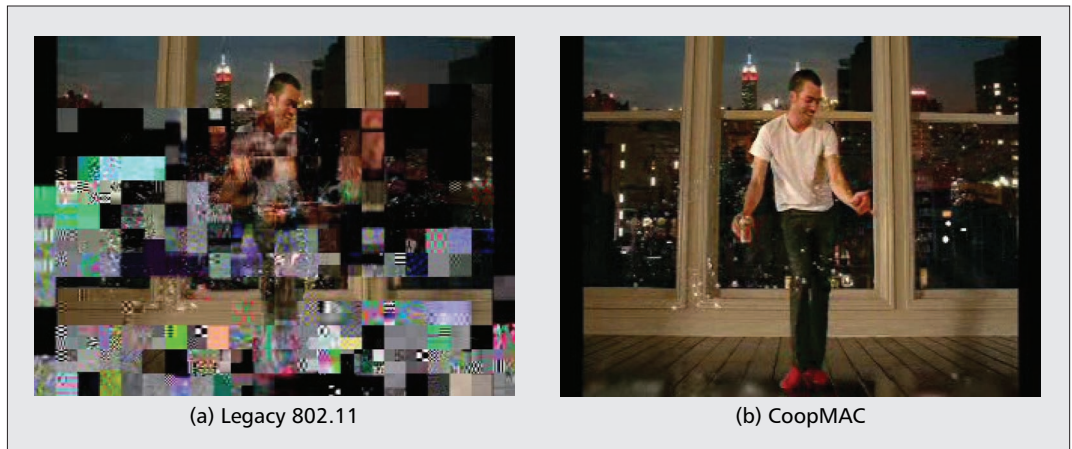
■ Figure 4. Open source drivers demo snapshot: a) legacy 802.11; b) CoopMAC.
