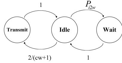
Fig. 2: Discrete Markov Chain Model
