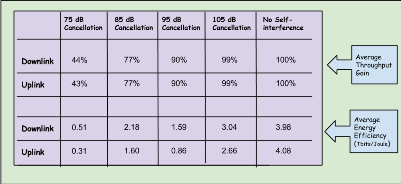
Figure 5. Average throughput gain and energy efficiency (terabits per joule) with full duplex UEs.
