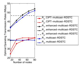
Figure 4: Average transmission rates vs number of nodes for different transmission schemes.
