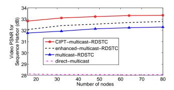
Figure 3: Achievable PSNR of Video Sequence Harbor vs number of nodes for different transmission schemes.
