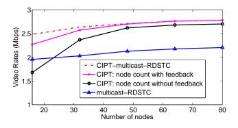
Figure 5: Video rates vs number of nodes for *CIPT*multicast-RDSTC node count case with and without feedback, and comparison to multicast-RDSTC (which does not require feedback).
