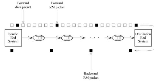
Fig. 5. A feedback-based flow control mechanism.
