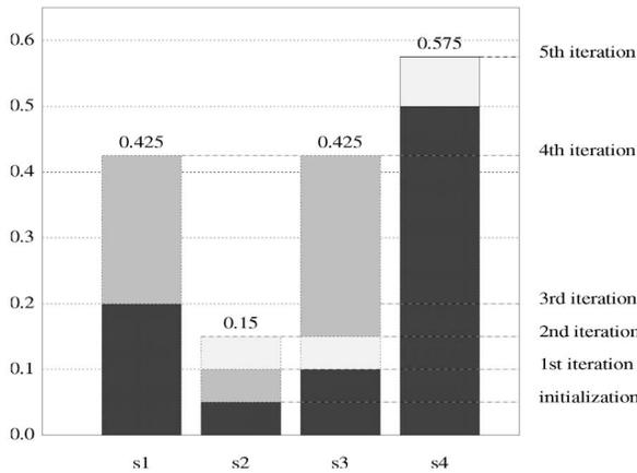
Fig. 4. Graphical display of rate allocation for each flow at each iteration in the three-node network.
