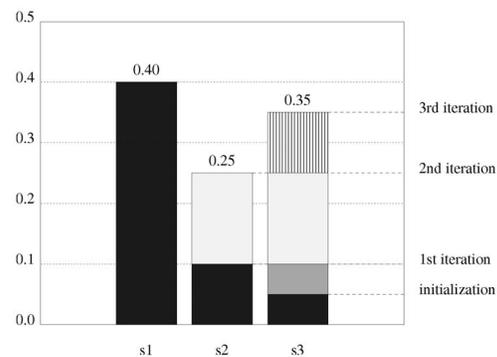
Fig. 2. Iterative steps in rate allocation as a “water-filling” process.
