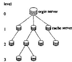
Fig. 1. An example of a hierarchical caching system based on tree topology.
