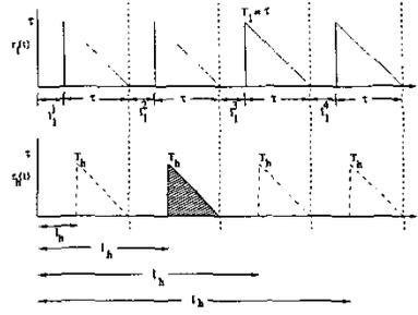
Fig. 3. A sample path of the TTL behavior of a cache server at level  $h$  in reference to the TTL behavior at level 1.
