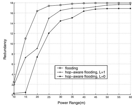
Fig. 3. The redundancy for different power ranges.
