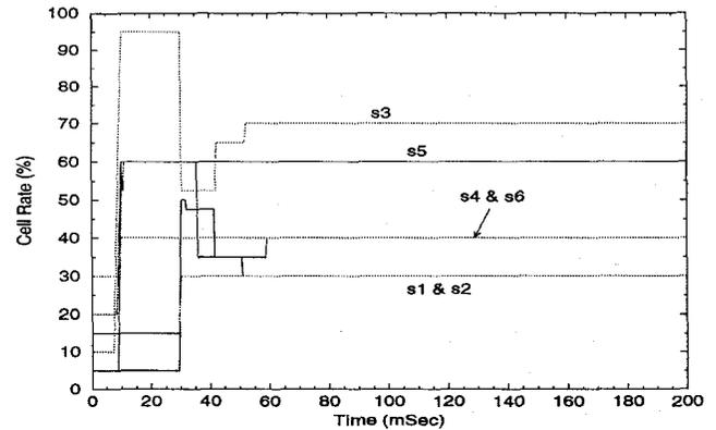
Figure 7: The cell rates of all connections for the MCRadd policy in the generic fairness network configuration.
