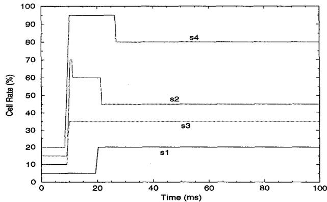
Figure 5: The cell rates of all connections for the MCRadd policy in the three-node network configuration.
