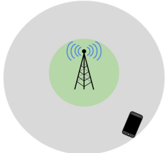
Fig. 1: Due to highly directional transmissions, millimeter wave (mmWave) systems will exhibit a large disparity in the cell range in omnidirectional communication (green) vs. directional (gray). If cell search does not exploit this antenna gain, mobiles in the outer gray area may be capable of high data rates, but not able to locate the base station to establish the communication.
